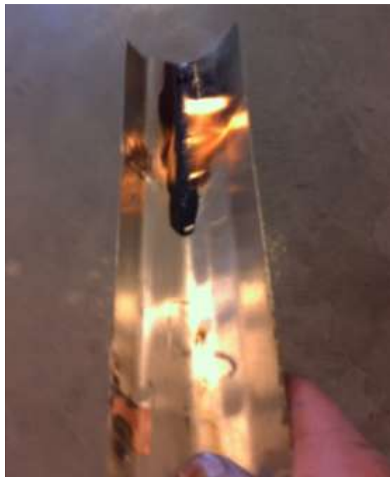
Bio-oil collected from the pyrolysis process (left). It can ignite, confirming its potential as a fuel (right).
