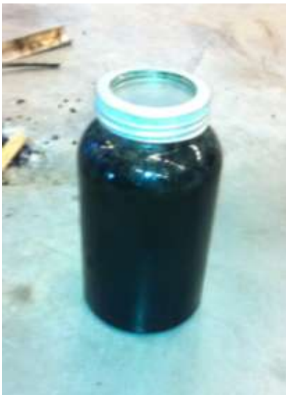
Bio-oil collected from the pyrolysis process (left). It can ignite, confirming its potential as a fuel (right).
