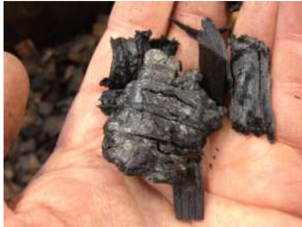
Bio-char produced in the prototype plant. The waste wood has been fully pyrolysed, leaving light carbonized chips
